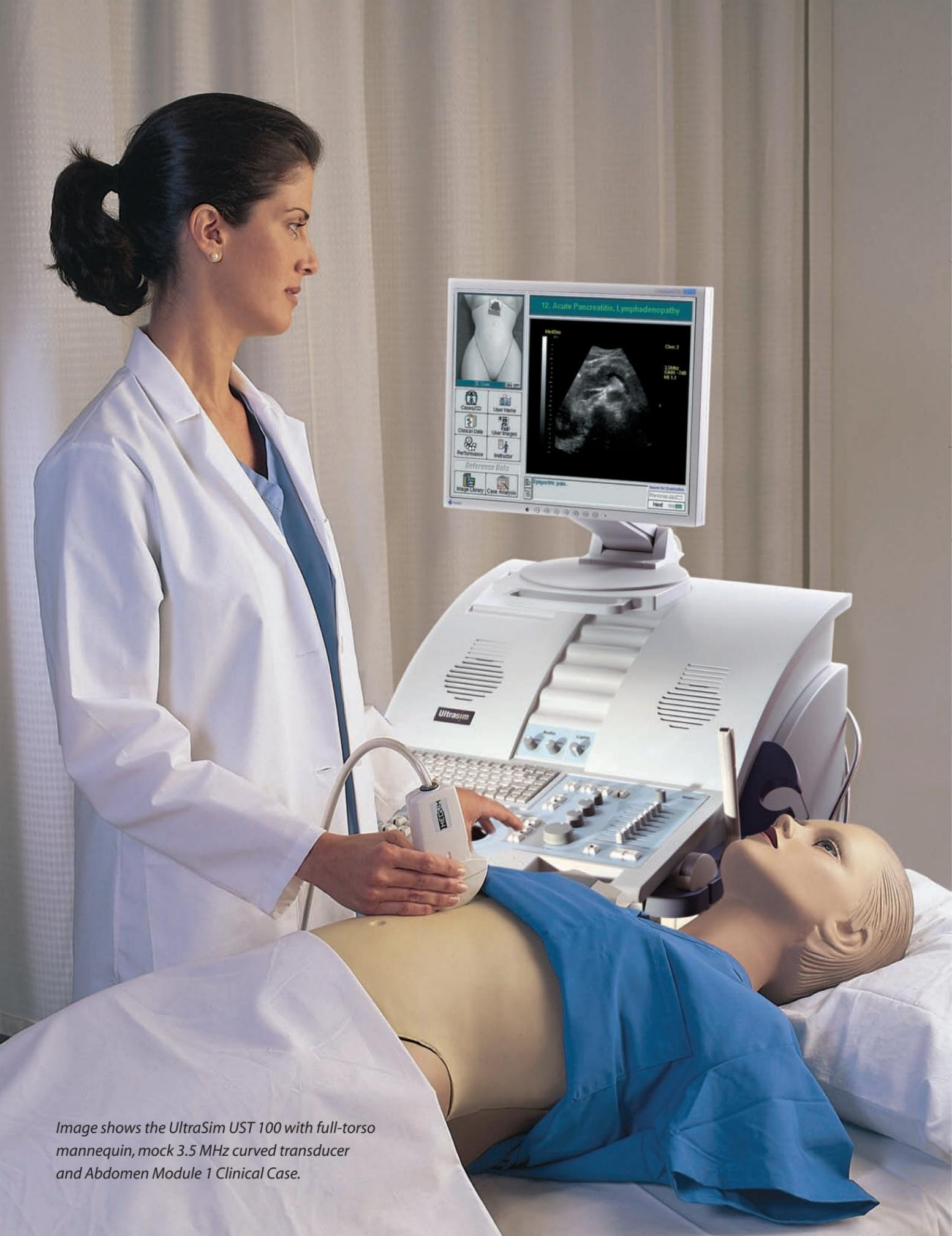
Image shows the UltraSim UST 100 with full-torso mannequin, mock 3.5 MHz curved transducer and Abdomen Module 1 Clinical Case.
